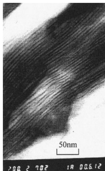
Figure 2 TEM image of a composite containing 3 wt % organic clay.
